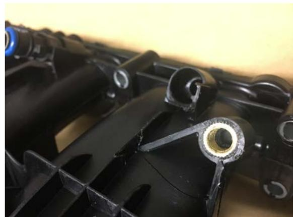
25. Secure the supplied injector port prep tool into a drill firmly so that it cannot spin inside the drill chuck. With the drill in clockwise rotation drill down into the injector port until the tool stops going down. Stop drilling and without removing the tool from the manifold disconnect the drill from the injector prep tool.
