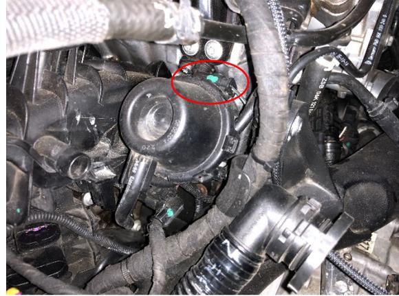
41. Route the provided wire harness along the same path of the factory harness down the driver side of the engine. Continue routing the wiring along this path until it reaches the ECU. Secure the wire as you go with tie wraps.
