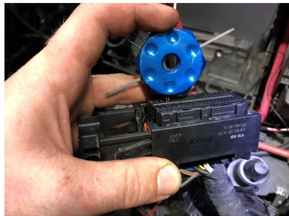
46. While removing the terminal blanks from the 105 pin connector you noticed they each face a certain direction this locks them in place in the connector when the purple locking slide in installed.
