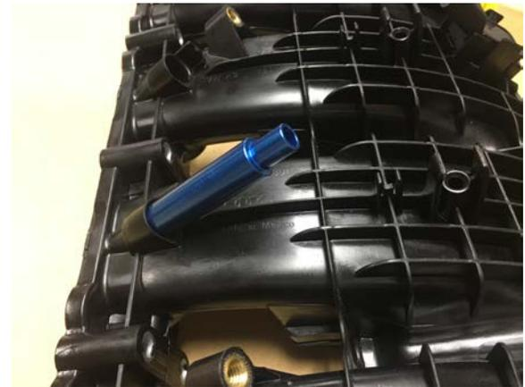
26. Tighten the supplied 7mm drill bit where just the end of the bit is in the chuck of the drill (the bit is just long enough to go through the port). Then drill through the center of the injector port prep tool using high speed on the drill bit and minimal force until the bit passes through the inside of the intake manifold. Repeat steps 24 & 25 for the remaining 3 holes.
