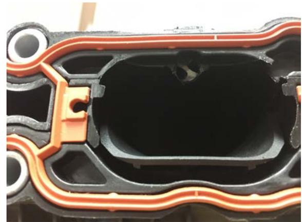
27. Using a rotary tool grind back any uneven plastic and burr's on the inside of the intake manifold from the drilling process. The O-ring seal is far back inside of the injector port so you can remove quite a bit of material here to make a nice smooth flow for the air and also remove any potential plastic from altering injector spray pattern.
