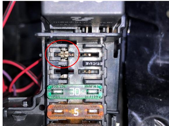
54. Reinstall the fuse panel into the fuse box pushing aligning each of the T shape alignment tabs on the box with the fuse panel. The panel should lock back in place just as it was previously. Install a 20amp fuse in this new fuse location.
