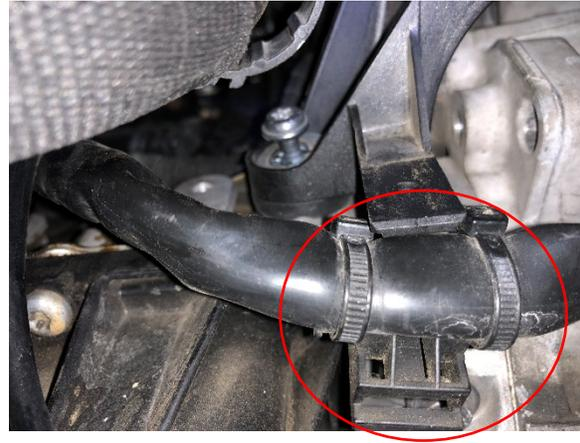
9. Unclip the harness connected to the turbo outlet pipe, and then disconnect the connector for the MAP sensor located on the throttle body inlet pipe.
