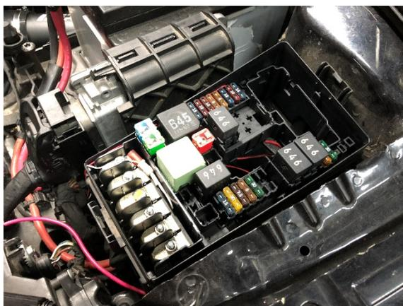
51. Remove the front cover of the fuse box by grasping the cover and pulling up to slide the cover off while releasing the locking tab.
