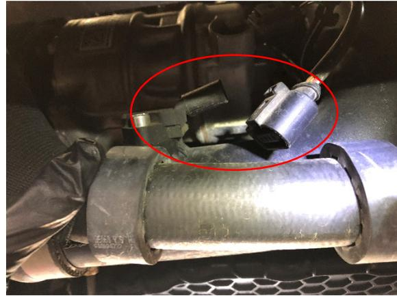
10. Remove the remaining T30 screw securing the throttle body inlet pipe. Disconnect the throttle body inlet pipe from the throttle body and let it hang down.
