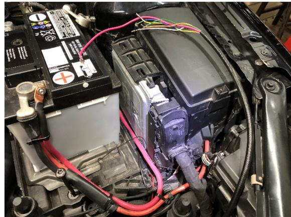
42. Disconnect the 105 pin connector from the ECU located next to the battery and fuse panel by flipping the lever on the back side of the connector down while lifting up on the tab on top of the connector.
