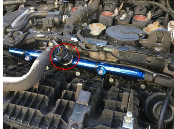
36. Reinstall the 10mm triple square bolt and 13mm nut to the support brace under the manifold. Tighten both hand tight first. Then once both are installed torque the 13mm nut followed by the 10mm triple square bolt.
