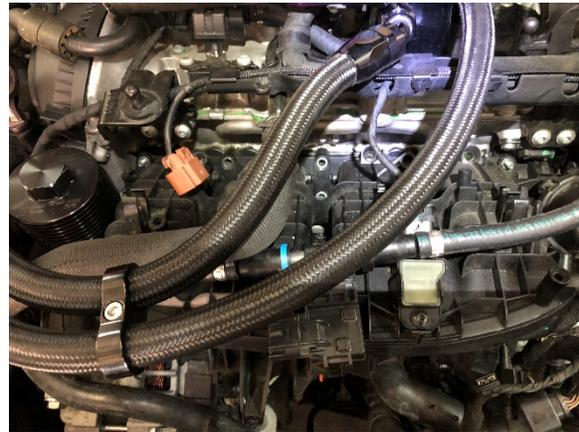
21. The 13mm bolt we loosened in step 16 is now the only thing securing the intake manifold to the car. Remove this nut and carefully pull the intake manifold back from the cylinder head rotating the passenger side up and slide the electrical connectors off their support bracket then remove the two T30 screws which secure the bracket to the manifold.
