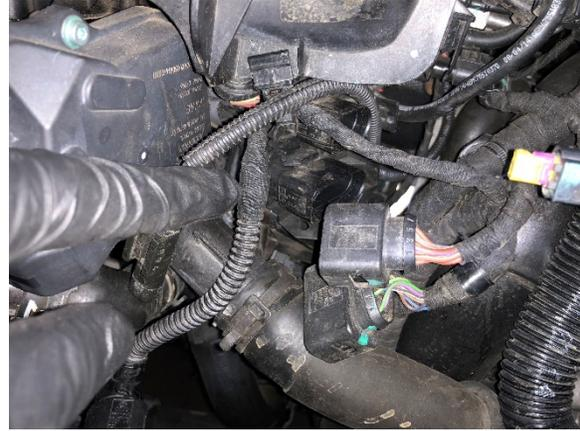
12. Disconnect the Intake manifold runner flap control valve and camshaft position sensor connectors located on the driver's side of the intake manifold & cylinder head.
