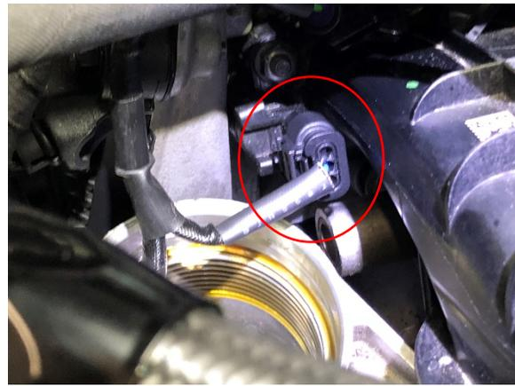
32. Connect each of the injector connectors working from passenger side of car to drivers side of car until all are connected.
