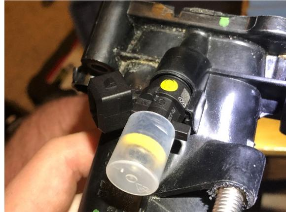
31. Remove the supplied harness from packaging and start at the opposite end of the Red wire. The two connectors (male female) connect to the factory intake runner flap position sensor. Connect the factory runner flap connector to the supplied harness and then plug the matching connector on the new harness into the runner flap position sensor.
