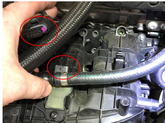
20. Remove the two 10mm nuts from the passenger side of the intake manifold. Then remove the eight T30 bolts securing the intake manifold to the cylinder head.
