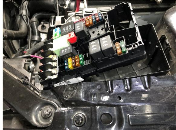
53. Once the fuse panel is removed from the box route the red wire through the box along with the factory wires. Then insert the metal terminal with red wire into the fuse panel in the location shown below.
