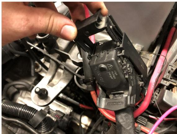
50. Remove the top cover from the fuse box. Then pull the tab at the front of the fuse box and lift the slide door as shown in the photos below.
