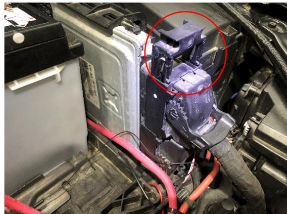
43. Ensure the lever on the connector is fully open. Then use a small screw driver to pry the cover and lever off the 105 pin connector as shown in the photos below.
